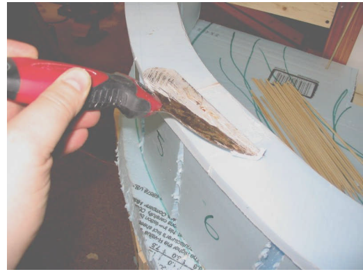
Photo 24 – Using the spackling compound makes it easy to fill gaps and correct small imperfections in adjoining subroadbed section
