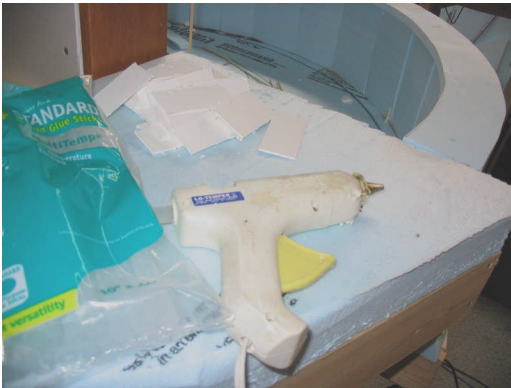
Photo 25 – I use illustration board for roadbed. It is attached to the subroadbed with a low-temperature hot-glue gun. After the glue sets, excess glue can be cut away with a hobby knife with a chisel blade. The roadbed is then sanded flat.
