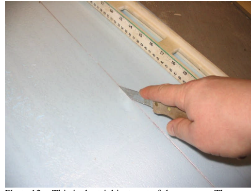
Photo 12 - This is the trickiest part of the process. The cut must be as close to perpendicular to the surface of the foam as possible. This makes track laying much, much easier
