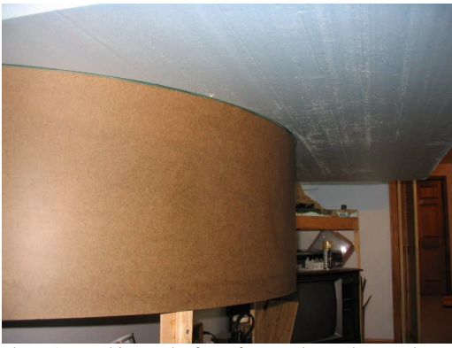
Photo 5 – Looking at the foam from underneath, a marker can be used to draw the needed outline.
