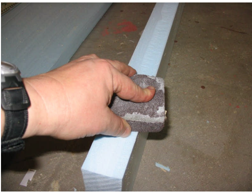
Photo 13 - Imperfections in the cut are sanded down to get a flat surface.
